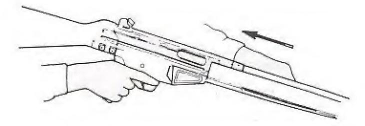
3. Check again to make sure the safety lever is on "S" or "Safe" position, then point the rifle in a safe direction. You may now cock the rifle by pulling the cocking lever rearward with your left hand and engaging it in the cocking lever notch.
